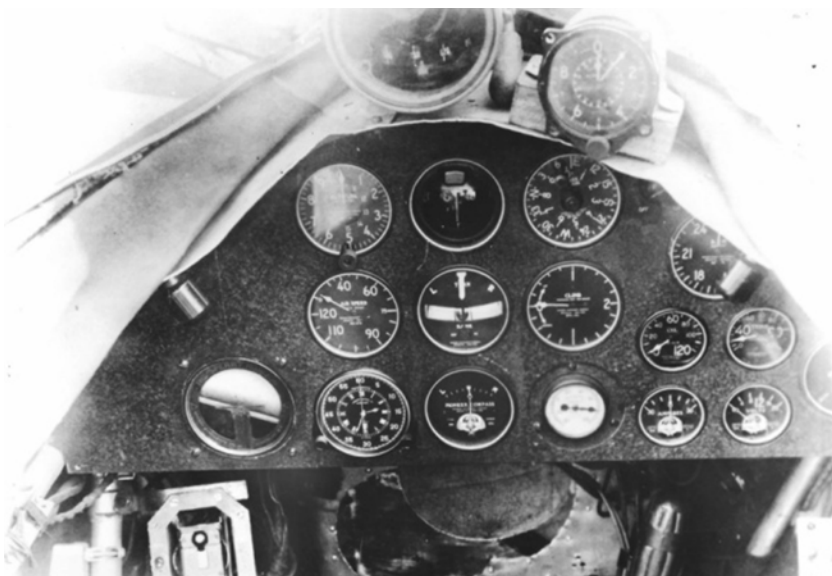
The Instrument Panel: The Kollsman altimeter is on the upper right. The radio beacon and direction finder from Radio Frequency Laboratory is the octagon-shaped device in the lower left hand corner and the Sperry artificial horizon is on the lower left of the bottom instruments row.
