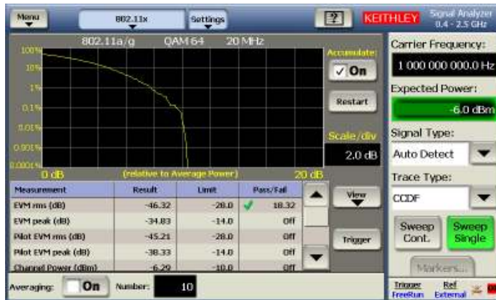
Figure 2. CCDF curve of 802.11A 64QAM signal - No Compression.
