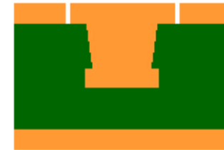
Laser Drilled Micro Via
