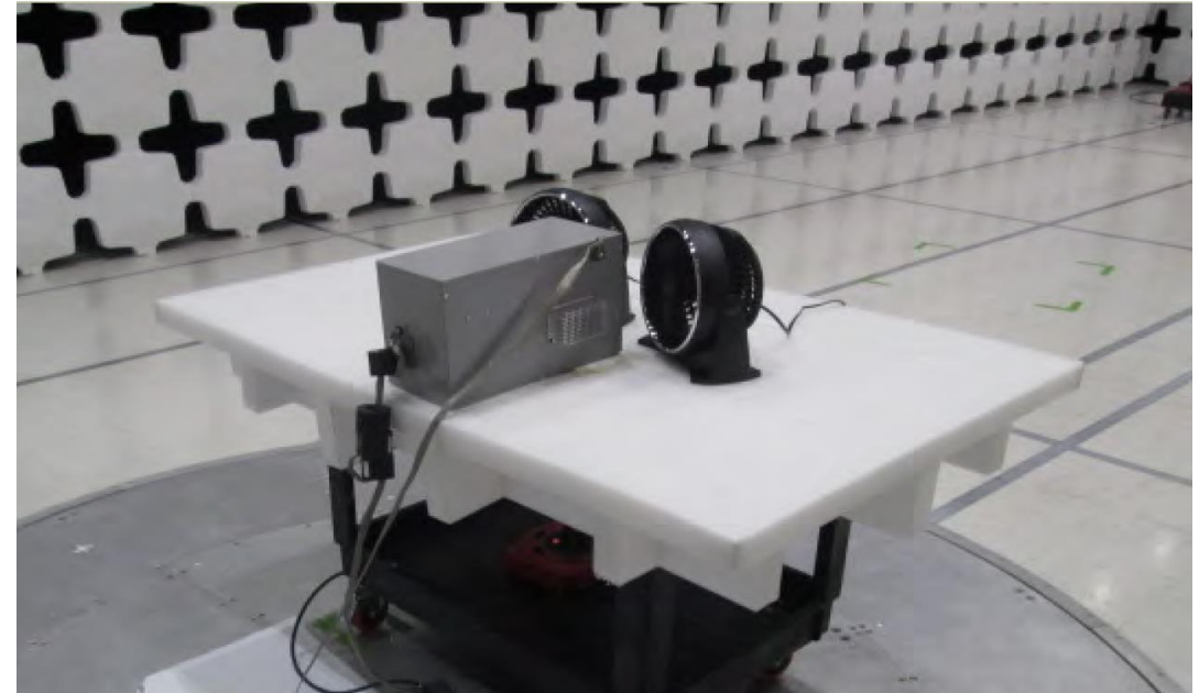
Radiated Emission Test Set-up
