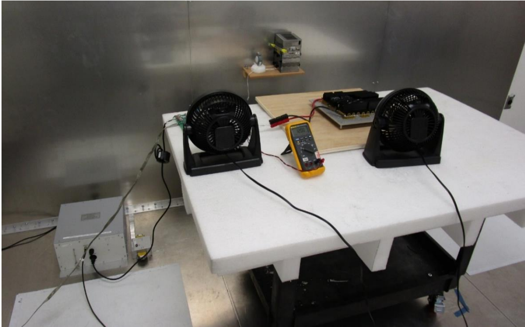
Conducted Emission Test Set-up
