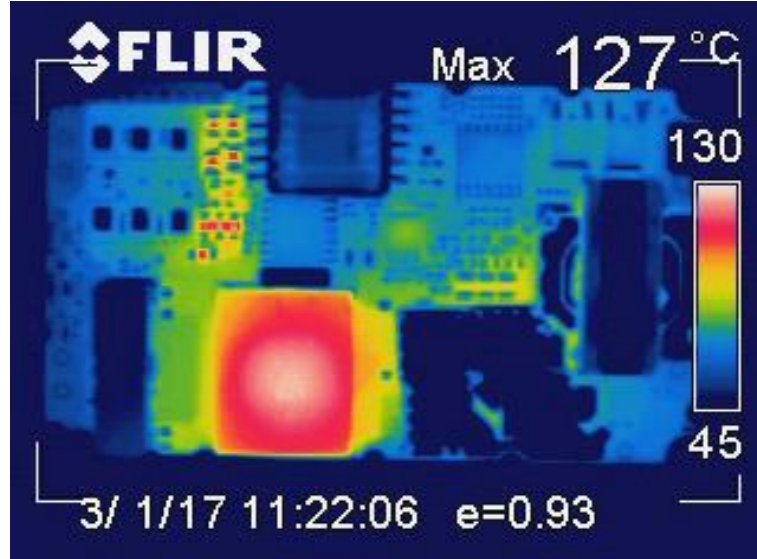
Open Frame Module, Tested in Socket V_{in}=230V_{ac} , I_o=18A , V_o=28V , P_o=504W
