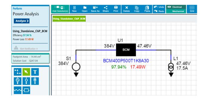
> Efficiency = 97.94% in forward direction at 384 V HI side voltage and 17.5 A LO side current
