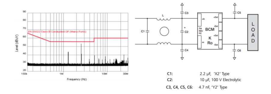
With high switching frequencies and a galvanic isolation barrier it is possible to return HF/VHF common mode noise currents back to the noise source with simple discrete filters
