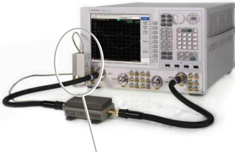
Agilent's unique noise-figure-calibration technique uses an ECal module as an impedance tuner to remove the effects of imperfect system source match
