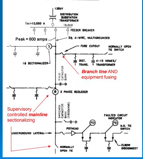
The generic distribution feeder is one which is designed radial and with one supply source....the substation circuit breaker, and using fuses on most, if not all, branch taps.
