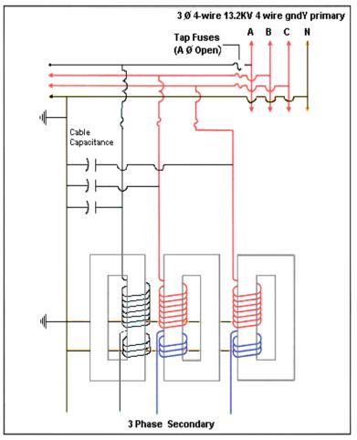
3 Phase primary grounded wye -- grounded wye triplex core transformer, with no ferroresonance induced in the dead phase (no magnetic flux currents)
