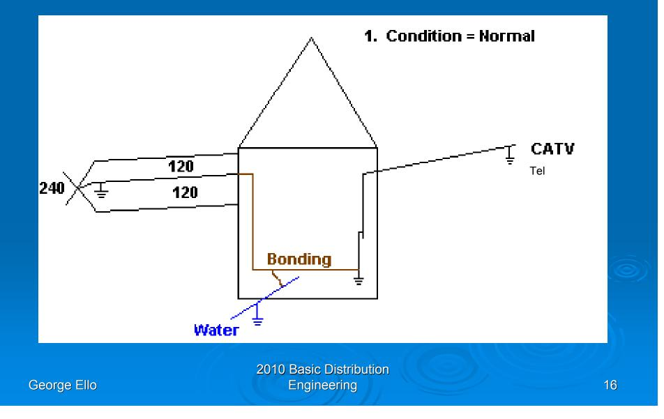
A 100% metallic "city" water system is an excellent ground system with multiple ground points. <u>Under normal conditions, it might carry up to 50% of house load</u> return current. Smaller fractions of current will use CATV and Tel paths.
