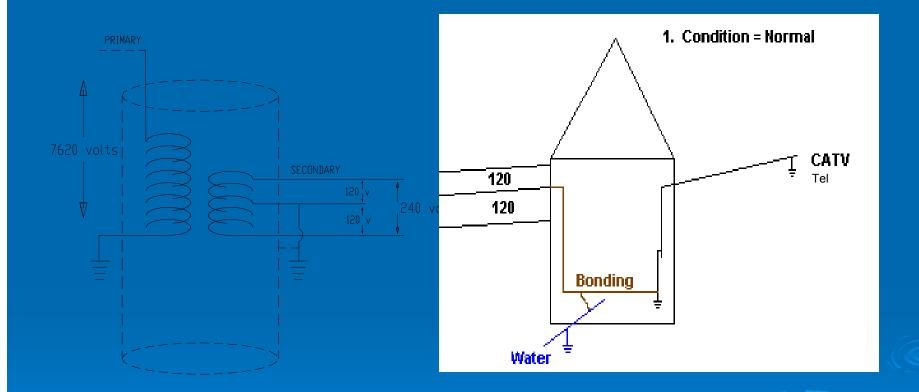
Such split-phase electric supply requires a well-connected neutral system. Inside buildings, per NEC, neutral and ground systems are isolated.
