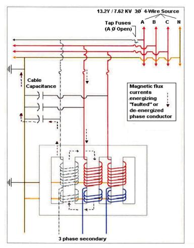
Primary side ferroresonance between cable capacitance and stray flux in a grounded wye -- grounded wye transformer.
