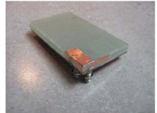
Dual port inverted PIFA
