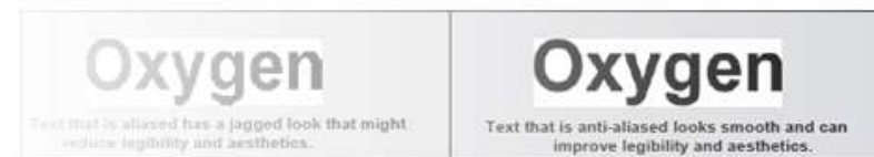
Figure 21.11—Comparison of normal text and anti-aliased text (reflecting font smoothing)
