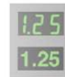
Figure 21.12—High-resolution displays should present information using optimized fonts (bottom) for maximum legibility rather than mimic lower-resolution displays like segmented LCDs (top)
