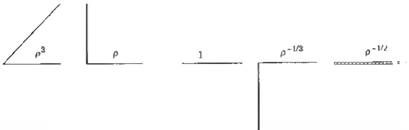
Figure 2.13 Variation of the surface-charge density (and the electric field) with distance \rho from the "corner" or edge for opening angles \beta = \pi/4, \pi/2, \pi, 3\pi/2, and 2\pi
