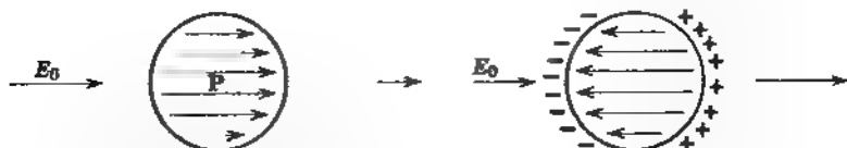
Figure 4.7 Dielectric sphere in a uniform field E_0 , showing the polarization on the left and the polarization charge with its associated, opposing, electric field on the right
