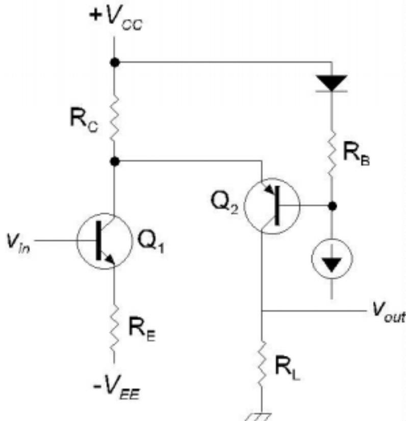
If current biasing is set so that both transistors operate statically at maximum power dissipation then, with a change in input voltage, each will move away from the maximum-power point of operation by approximately the same amount and the resulting thermal distortions will tend to cancel.
