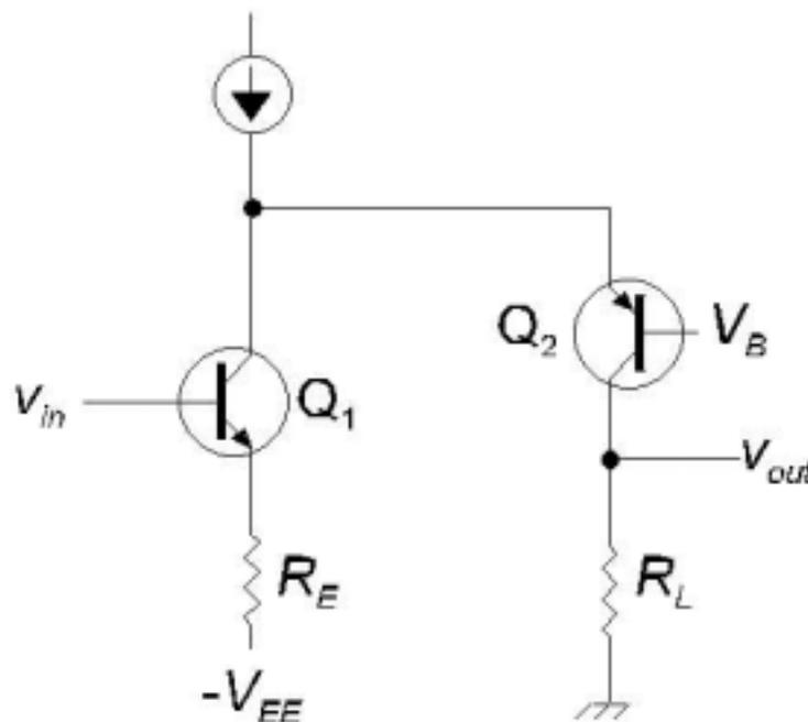
The cascode amplifier also provides voltage translation of the output to a higher static (dc) voltage than the input. This is not always advantageous, however, and can be eliminated by making the CB BJT of opposite polarity to the CE, as shown above.
