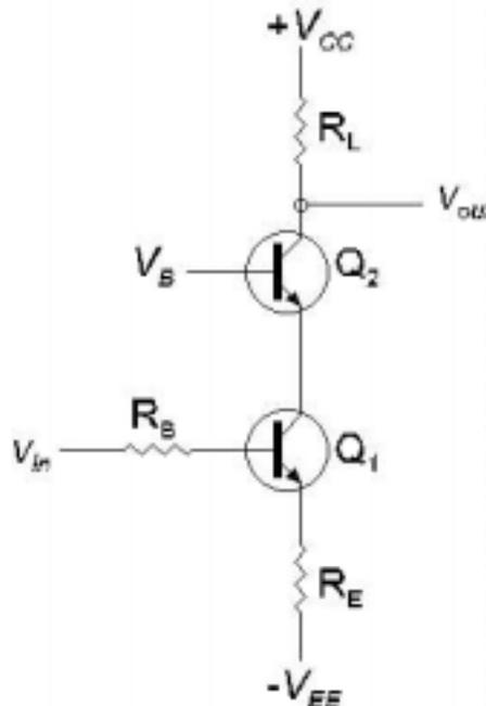
The basic cascode amplifier consists of an input common-emitter (CE) configuration driving an output common-base (CB), as shown above.
