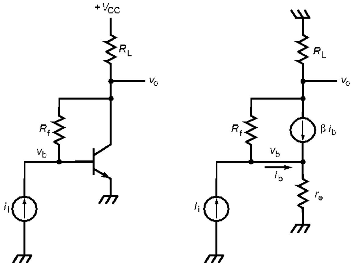
This amplifier will not be explained in detail here. (It is explained in more detail in *Analog Circuit Design*, available from <http://www.innovatia.com> ) It is a transresistance (current in, voltage out) amplifier, with a transresistance of:
