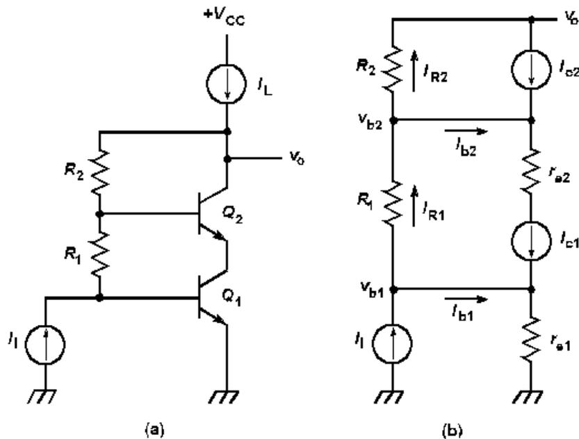
If speed is not the driving parameter, but voltage is, then this amplifier provides the advantage of dividing the collector voltage across two series BJTs. If  $R_1 = R_2$ , then each BJT need have only about half the breakdown voltage of a single-BJT amplifier. Again, the cascode shows an advantage for high-voltage applications.
