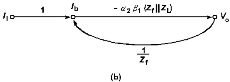
Finally, another shunt-feedback cascode variant uses a single feedback resistor, as shown above in (a), along with a flow graph (for feedback analysis) of the dynamic model of the circuit (b). ( $Z_f$  is  $R_f$  in parallel with  $C_f$  and  $Z_L$  is  $R_L$  in parallel with  $C_L$ .)  $C_f$  is added to provide an additional parameter for adjusting dynamic response. The transistor gain-bandwidth time constant,  $\omega_T$ , is related to  $f_T$  by:
